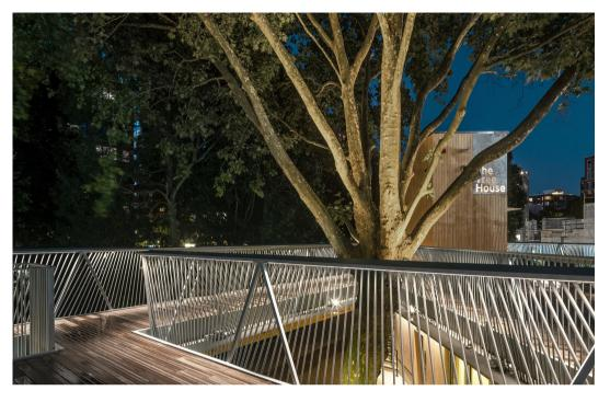
Light levels are kept low on the balustrades to allow views out over the park, while soft cross lighting to the tree creates a sense of theatre and supports an immersive experience on the roof deck.
