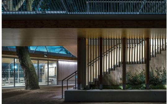
No light source is directed upward, and a warmer 2700K colour temperature is used, not only to support a relaxing experience but also to limit any impact on wildlife and the ecosystem.
